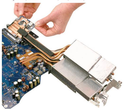
3. When handling the video card, hold it by the heat pipe brace as demonstrated on the iMac (24-inch) video card.
